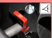
Engine is running but machine is not moving A Check setting of freewheel lever
