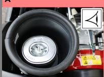
Engine is running erratically A Clean or replace air filter
